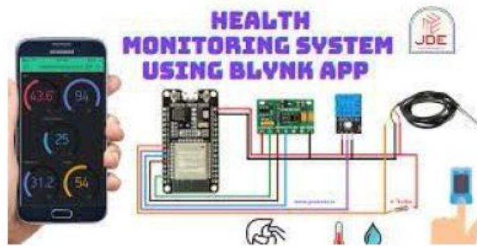
Fig. 5.1 CONNECTING SENSOR TO BLYNK IOT APPLICATION
