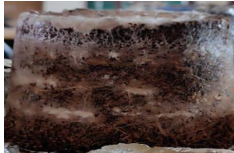
Figure 1 Mycelium Technology Brick Formation
